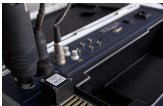
The GreenLine 8000 uses a wireless communication between MCU and RCU
